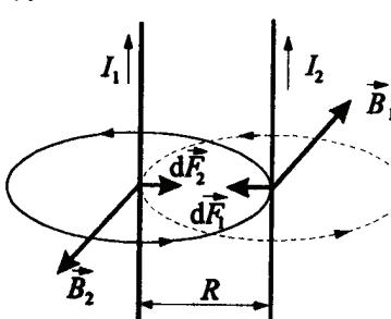
$$B_1 = \frac{\mu_0 \mu}{4\pi} \frac{2I_1}{R}, \quad dF_1 = I_2 B_1 dl.$$
