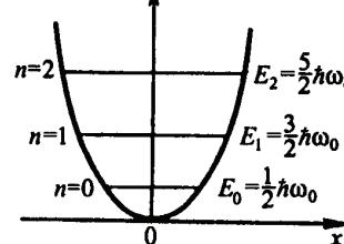
$$\frac{\partial^2 \psi}{\partial x^2} + \frac{2m}{\hbar^2} \left( E - \frac{m\omega_0^2 x^2}{2} \right) \cdot \psi = 0$$
